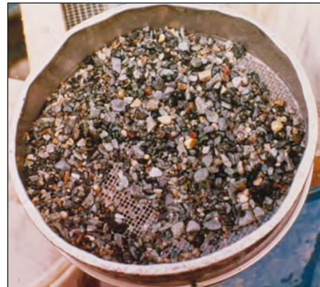
+10 mesh on screen for logging
